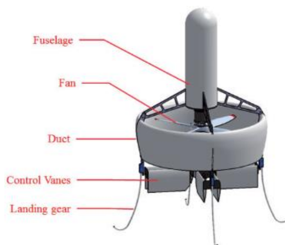
Fig. 1. ducted fan details
