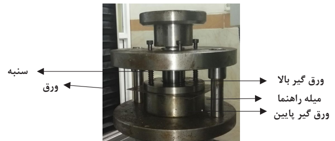
Fig. 7. The out of plane Nakazima test setup.
