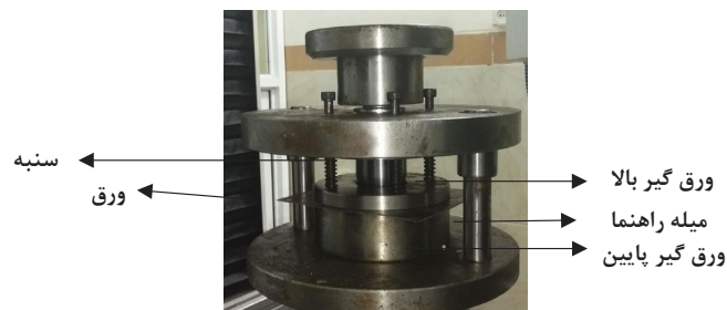
Fig. 7. The out of plane Nakazima test setup.
