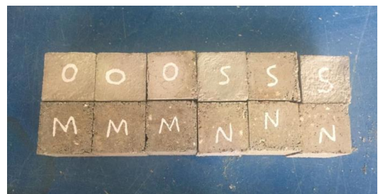
Fig. 2. Specimens for compressive strength test
