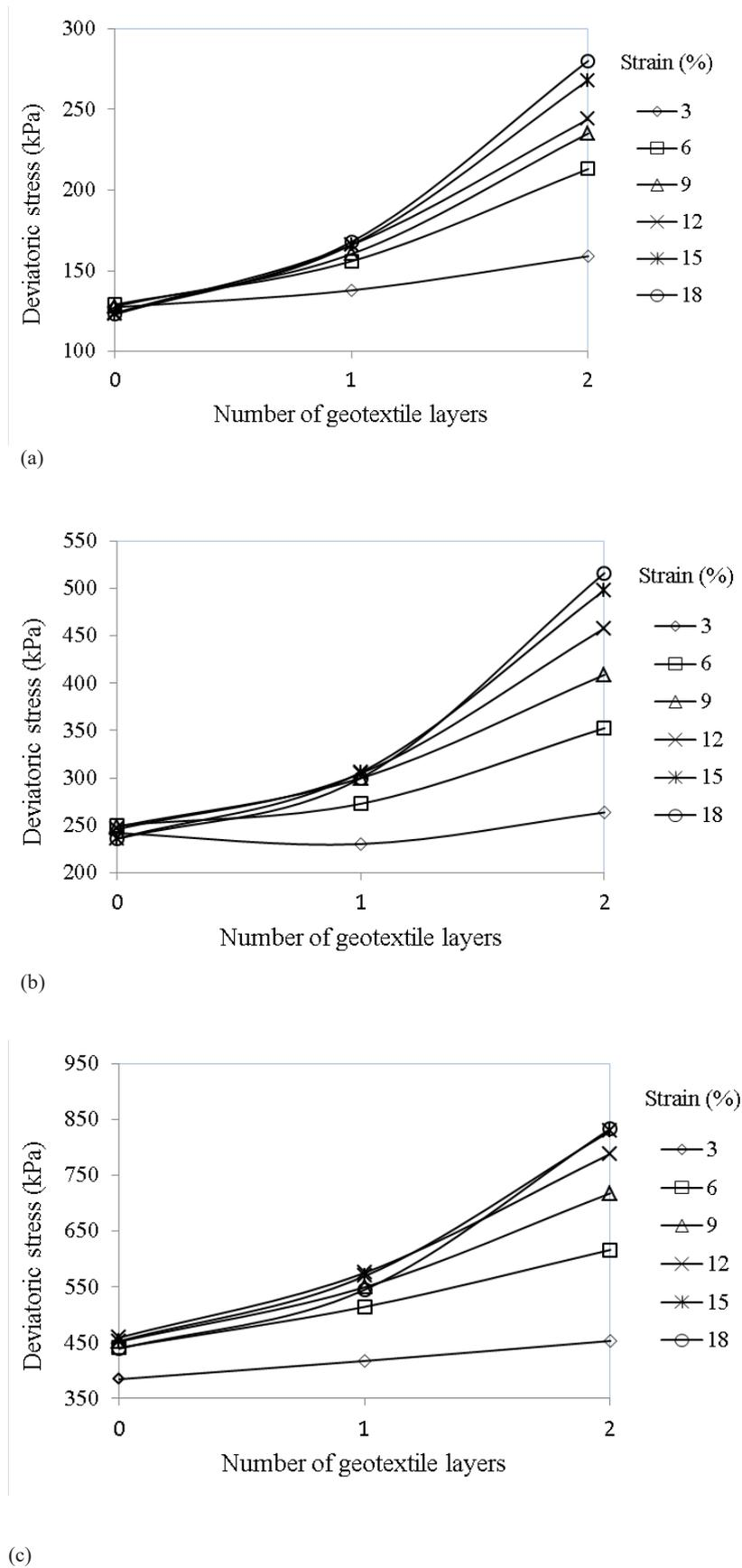
Fig. 9. Deviatoric stress values versus number of reinforcement at different strain levels under various confining pressure (a) 50 kPa; (b) 100 kPa and (c) 200 kPa
