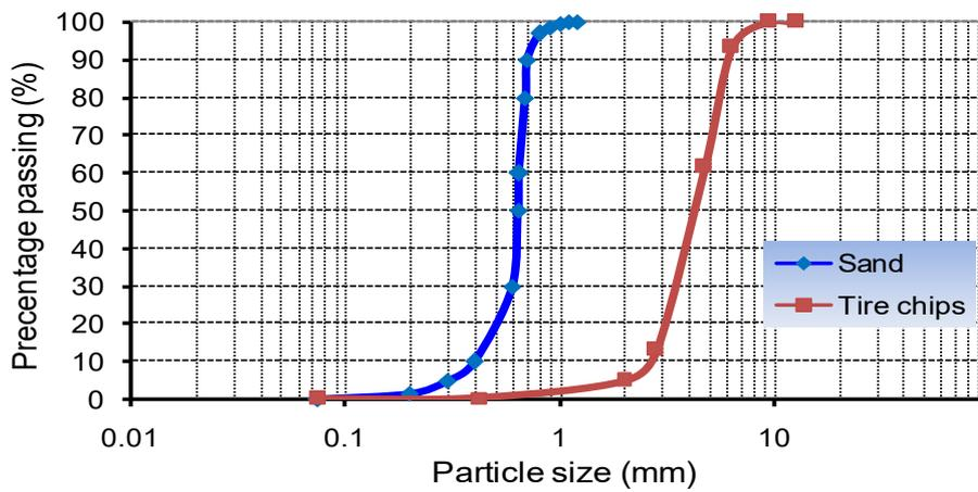
Fig. 1. Grain size distribution of sand and tire chip
