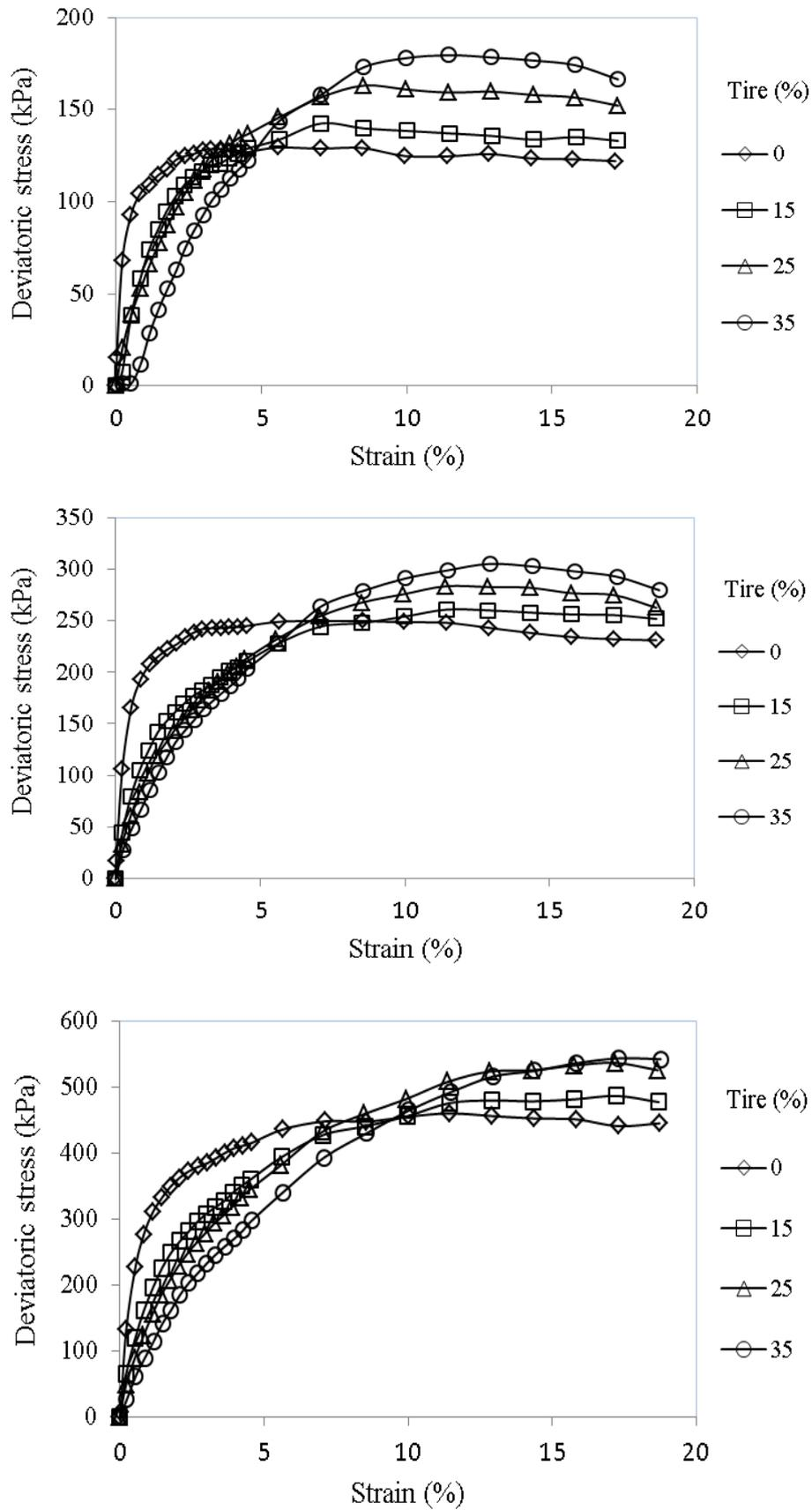
Fig. 6. Stress-axial strain curves for tire chip-unreinforced sand mixtures under various confining pressure (a) 50 kPa; (b) 100 kPa; and (c) 200 kPa
