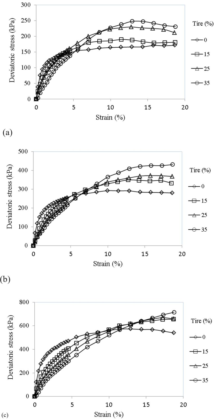
**Fig. 7. Stress-axial strain curves for tire chip-reinforced sand with one layer of geotextile under various confining pressure (a) 50 kPa; (b) 100 kPa; and (c) 200 kPa**
