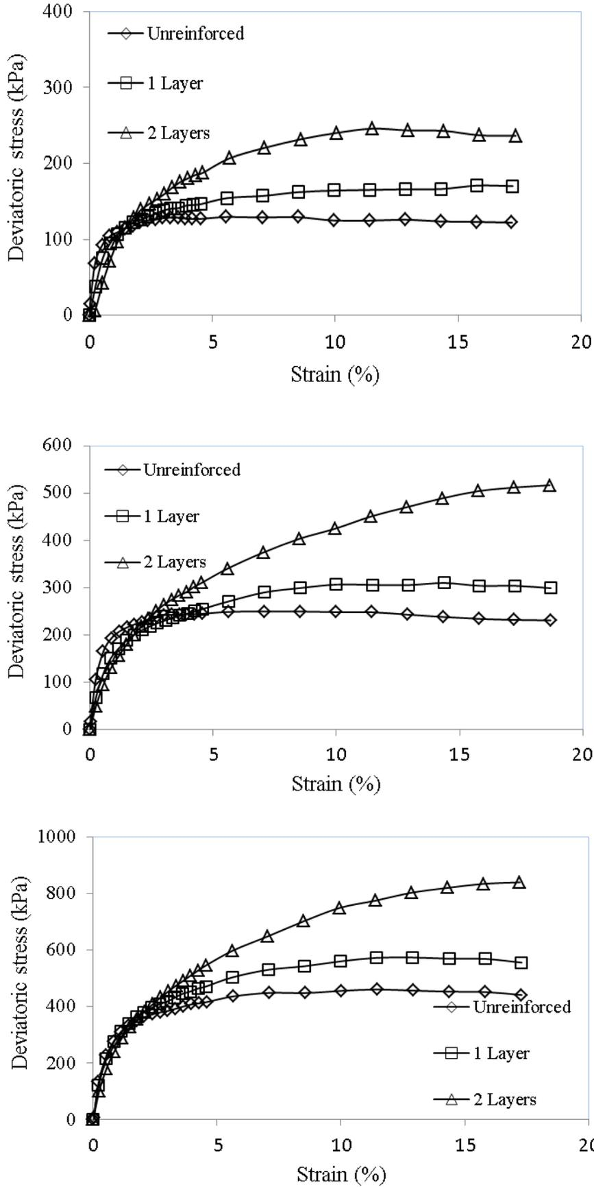
Fig. 5. Stress-axial strain curves for reinforced and unreinforced sand under various confining pressure (a) 50 kPa; (b) 100 kPa; and (c) 200 kPa
