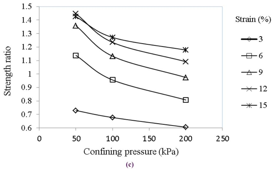
Fig. 14. Strength ratio values versus confining pressure at different strain levels and for various tire chip contents: (a) 15%; (b) 25% and (c) 35%
