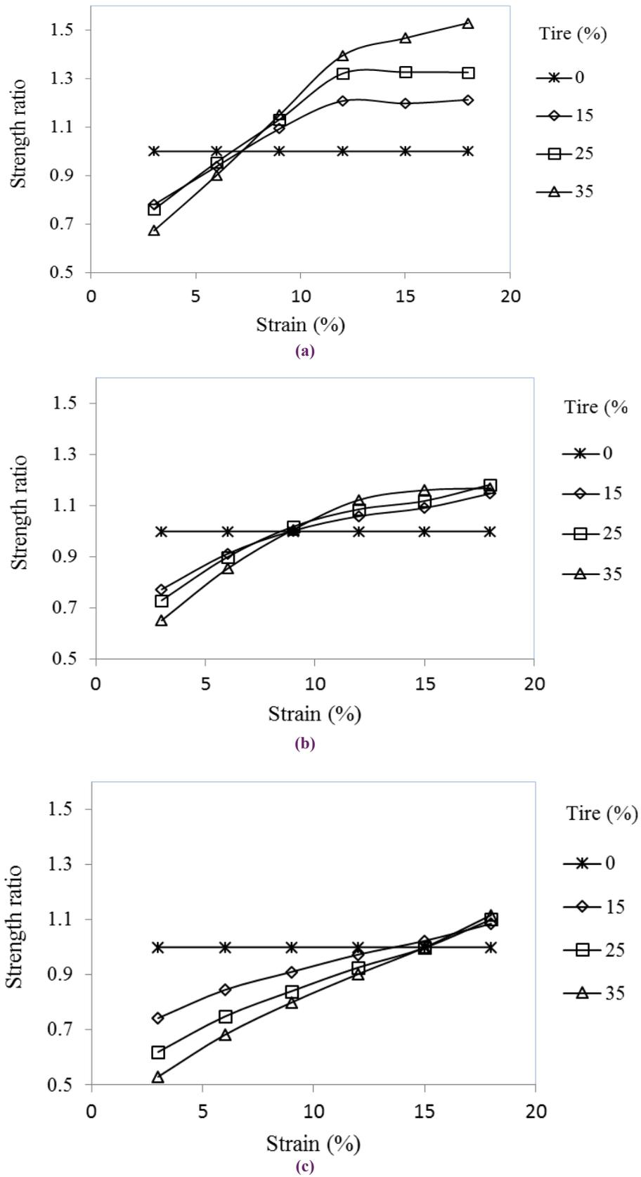
**Fig. 13. Strength ratio values versus axial strain for tire chip-reinforced sand with two geotextile layers under various confining pressure (a) 50 kPa; (b) 100 kPa; and (c) 200 kPa**
