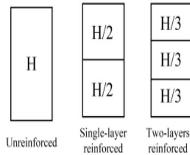
**Fig. 3. Geotextile arrangements for triaxial tests**
