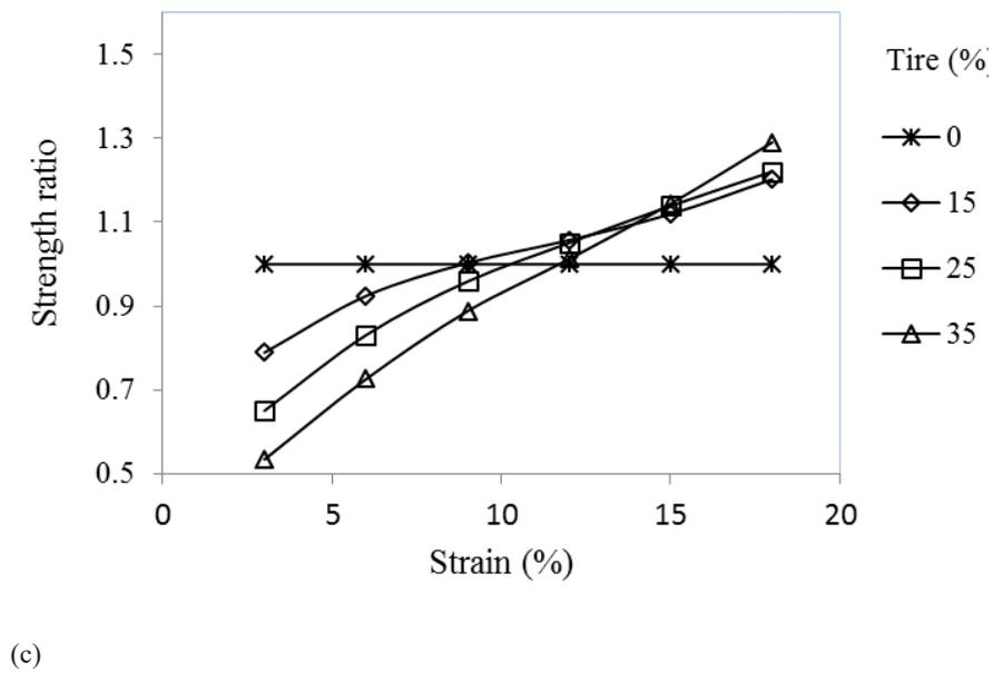
**Fig 12. Strength ratio values versus axial strain for tire chip-reinforced sand with one layer of geotextile under various confining pressure (a) 50 kPa; (b) 100 kPa; and (c) 200 kPa**
