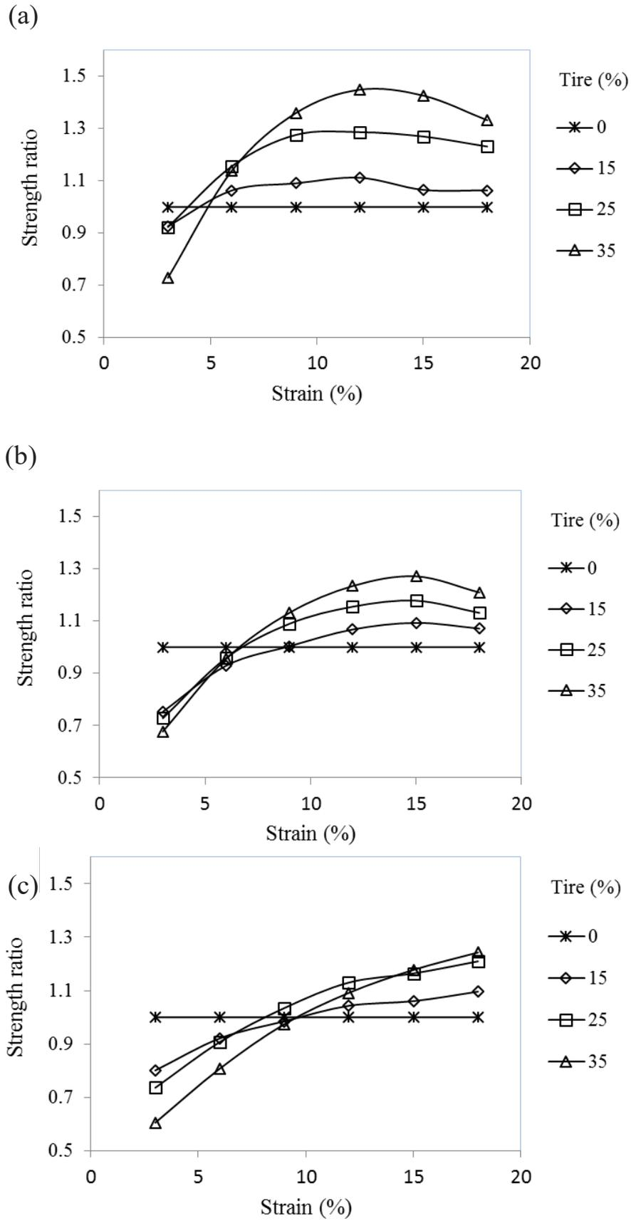
**Fig. 11. Strength ratio values versus axial strain for tire chip-unreinforced sand mixtures under various confining pressure (a) 50 kPa; (b) 100 kPa; and (c) 200 kPa**
