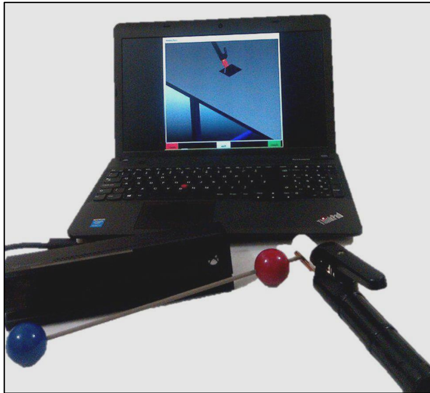
Fig. 13. Elements of the welding simulator
