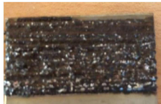
Fig. 17. The cross section of coated layer with optimal parameters. laser power 163 W, laser relative velocity 3 mm/sec and volume weigh of TiC 8.7374%
