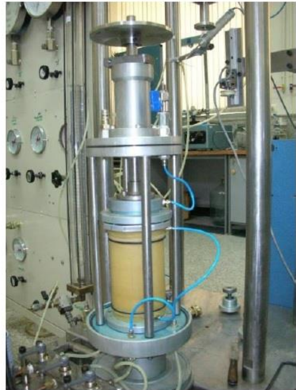
Fig. 6. Schematic diagram of hollow cylinder torsional apparatus (HCTA) and a specimen in the test using HCTA.
