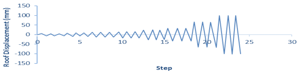
Fig. 2. Loading history for proof-of-concept test
