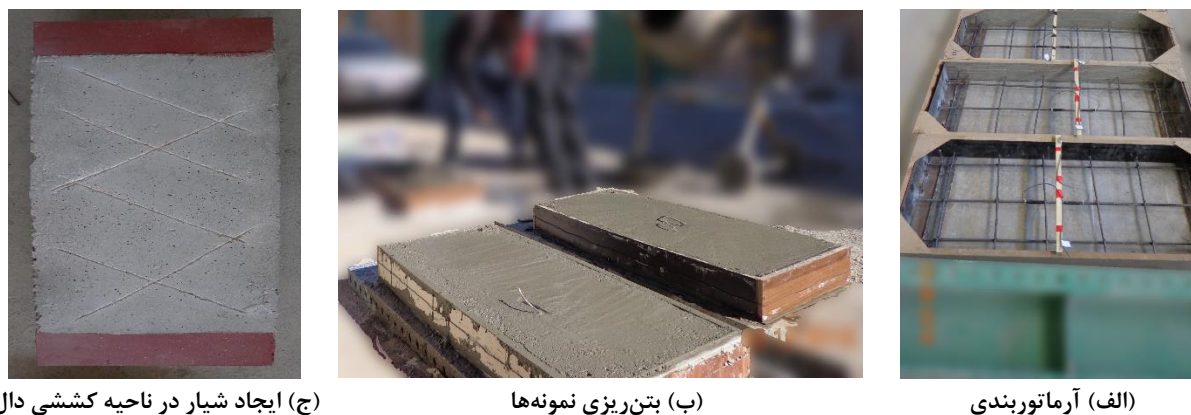
شکل ۱۰. نحوه‌ی ساخت دال‌های ضعیف Fig. 10. The manufacturing process of slabs specimens (a) slab's rebar installation (b) slab's concrete placement (c) slab's slotting
