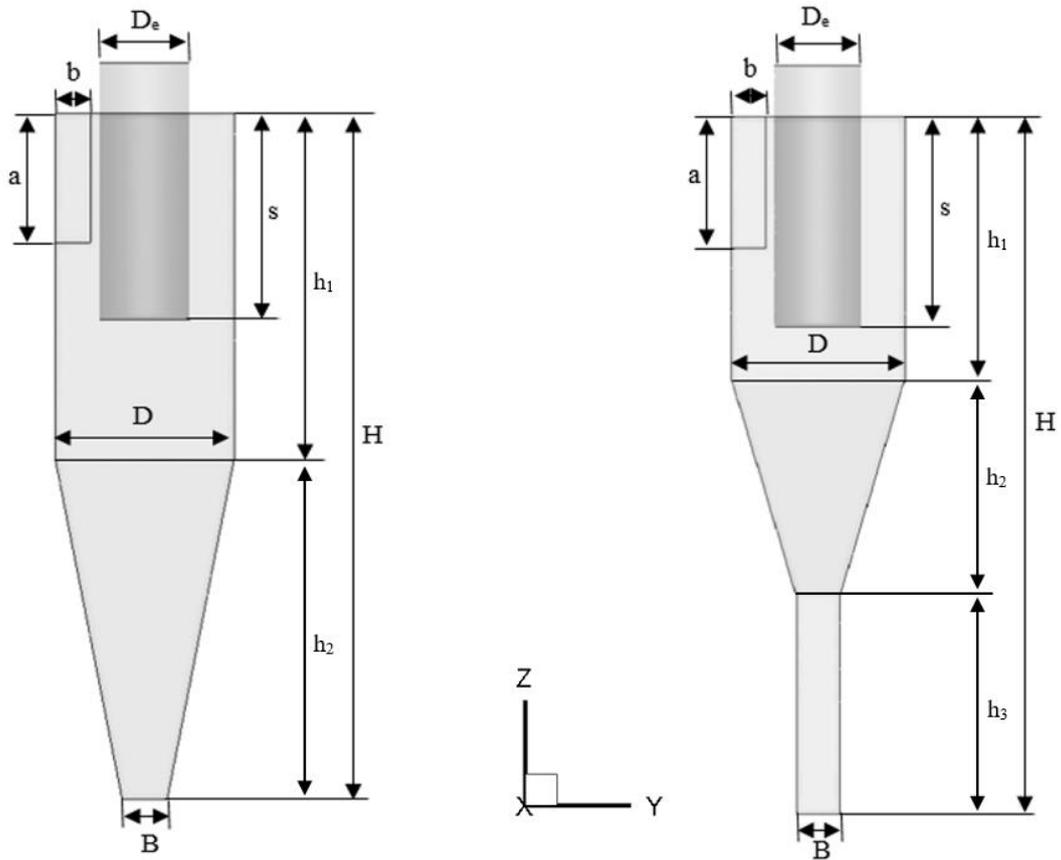
Fig. 2. Geometrical dimensions of square cyclone without dipleg (left) and with dipleg (right)
