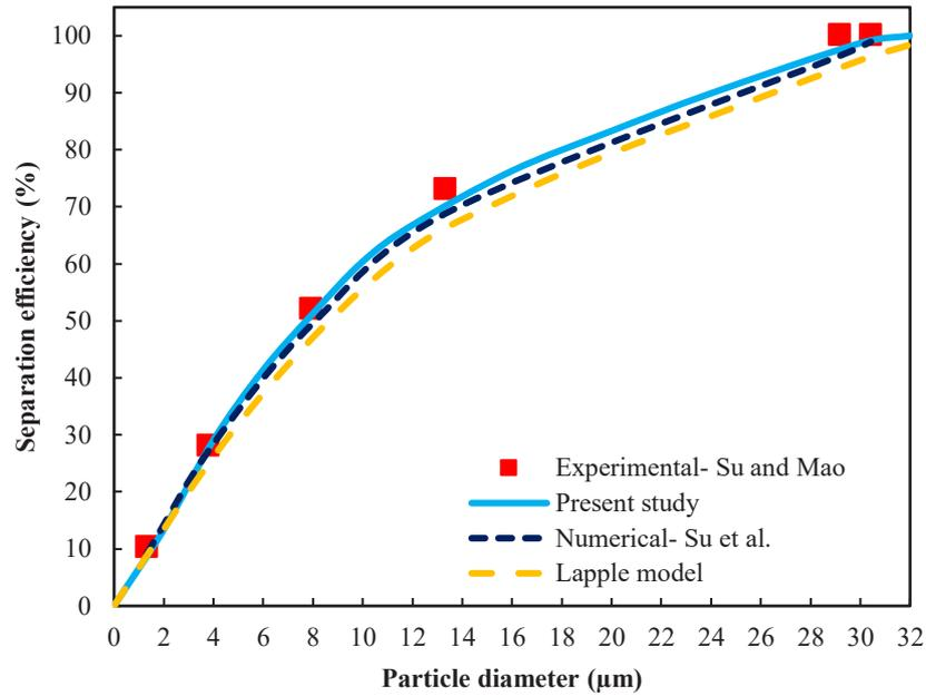
Fig. 6. Comparison between the separation efficiency of the present study and experimental data [25], numerical results [9], and the Lapple model [45] at  $v=20$  m/s
