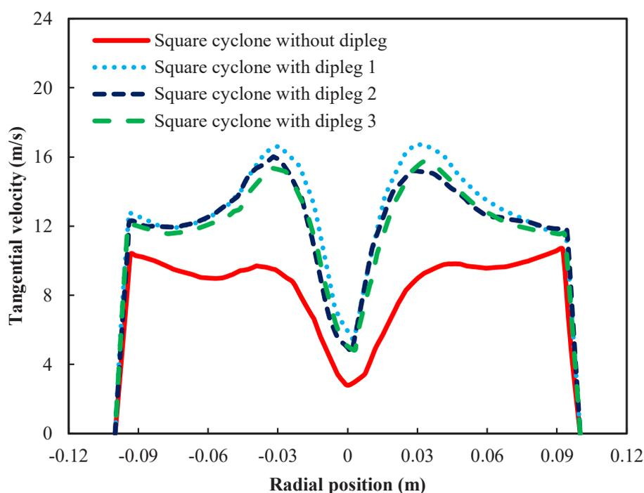
**Fig. 8. Comparison of tangential velocity distribution at location  $y=0.15$  m and  $v=12$  m/s**
