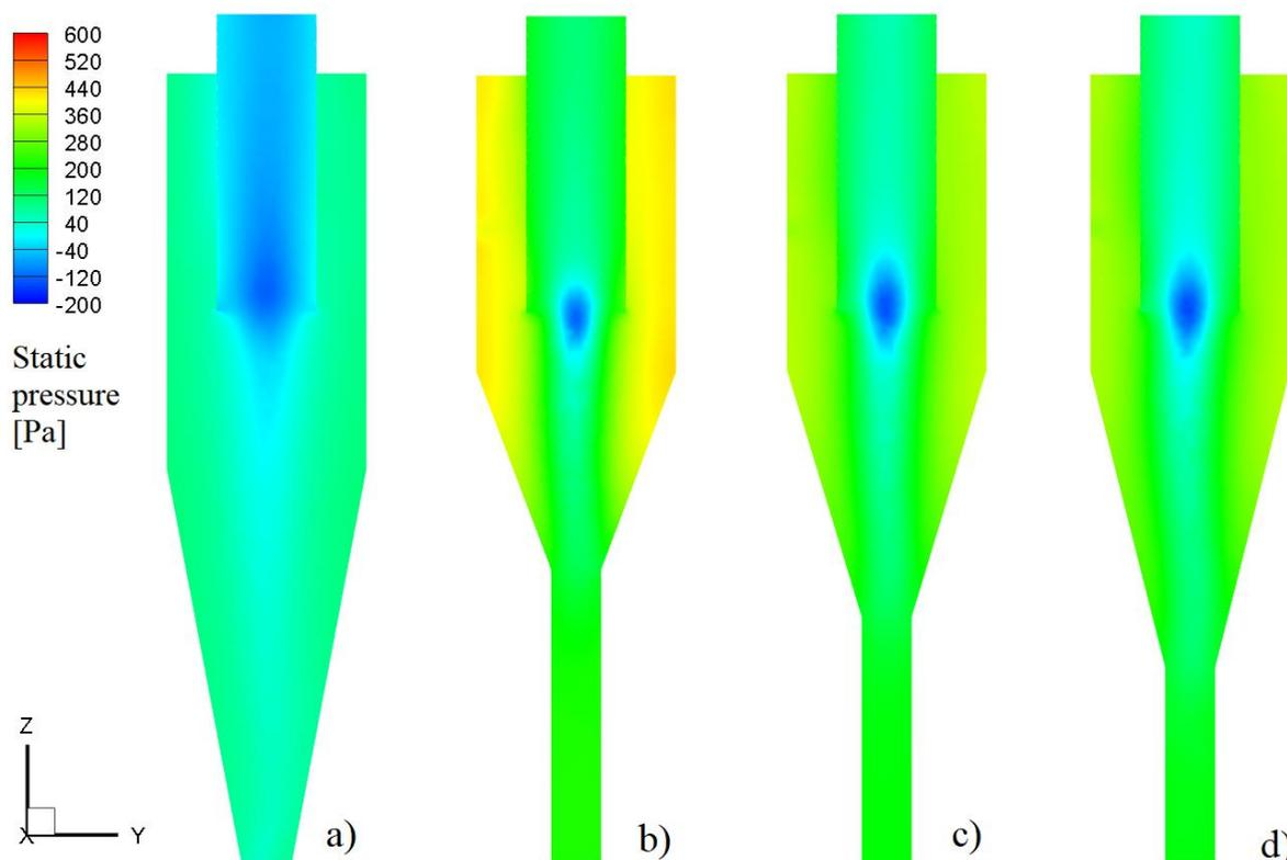
**Fig. 11. Contours of static pressure for square cyclone a) without dipleg b) with dipleg 1 c) with dipleg 2 d) with dipleg 3 at  $v=12$  m/s**
