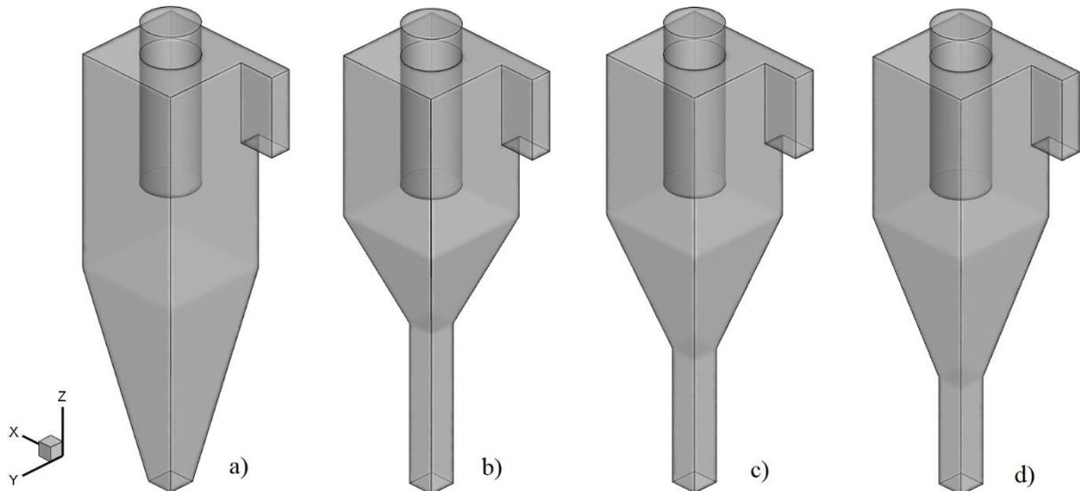
Fig. 1. Schematic view of a square cyclone a) without dipleg b) with dipleg 1 c) with dipleg 2 d) with dipleg 3
