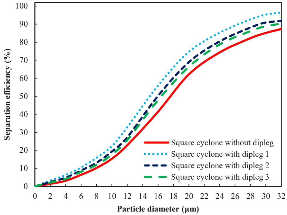
Fig. 9. Comparison between the separation efficiency of a square cyclone with and without dipleg at  $v=12$  m/s
