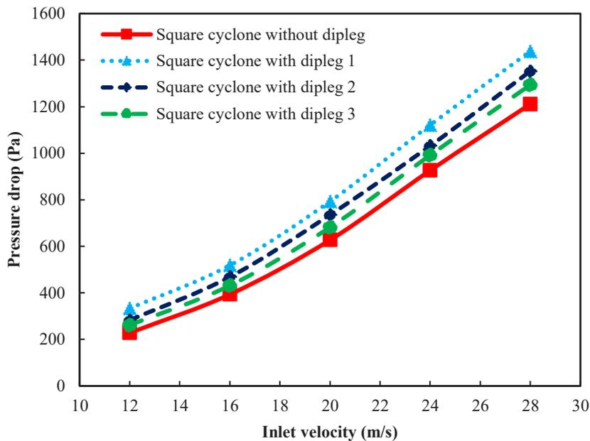
Fig. 7. The effect of inlet velocity on the pressure drop
