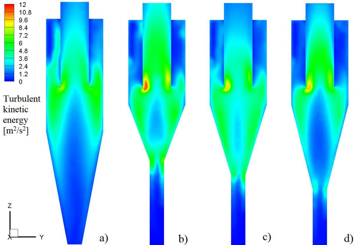
**Fig. 12. Contours of turbulent kinetic energy for square cyclone a) without dipleg b) with dipleg 1 c) with dipleg 2 d) with dipleg 3 at  $v=12$  m/s**
