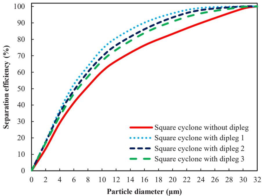
Fig. 10. Comparison between the separation efficiency of a square cyclone with and without dipleg at  $v=20$  m/s
