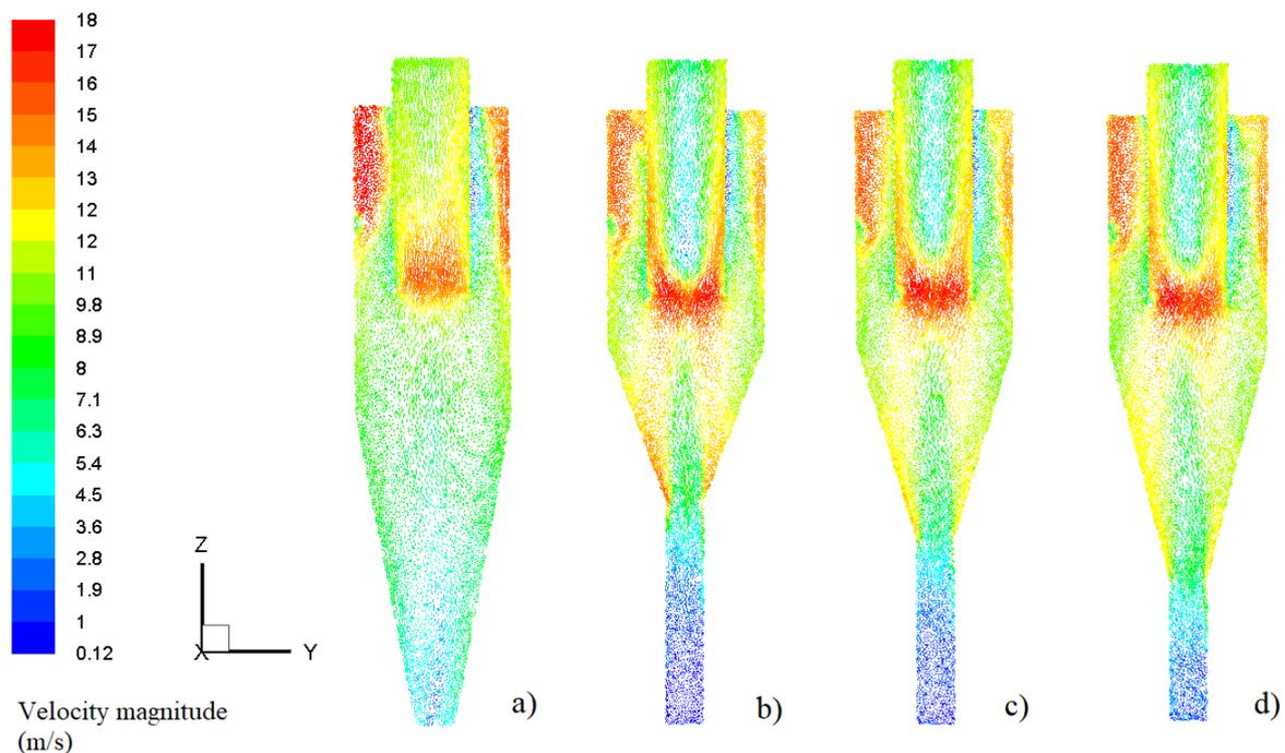
**Fig. 13. Velocity vector for square cyclone a) without dipleg b) with dipleg 1 c) with dipleg 2 d) with dipleg 3 at  $v=12$  m/s**
