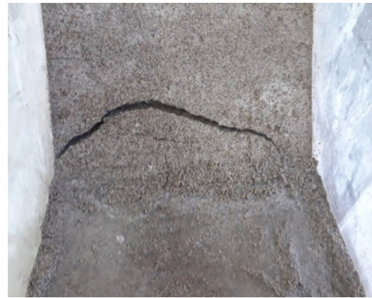
Fig. 3. Failure shape with 5% nano-lime covering
