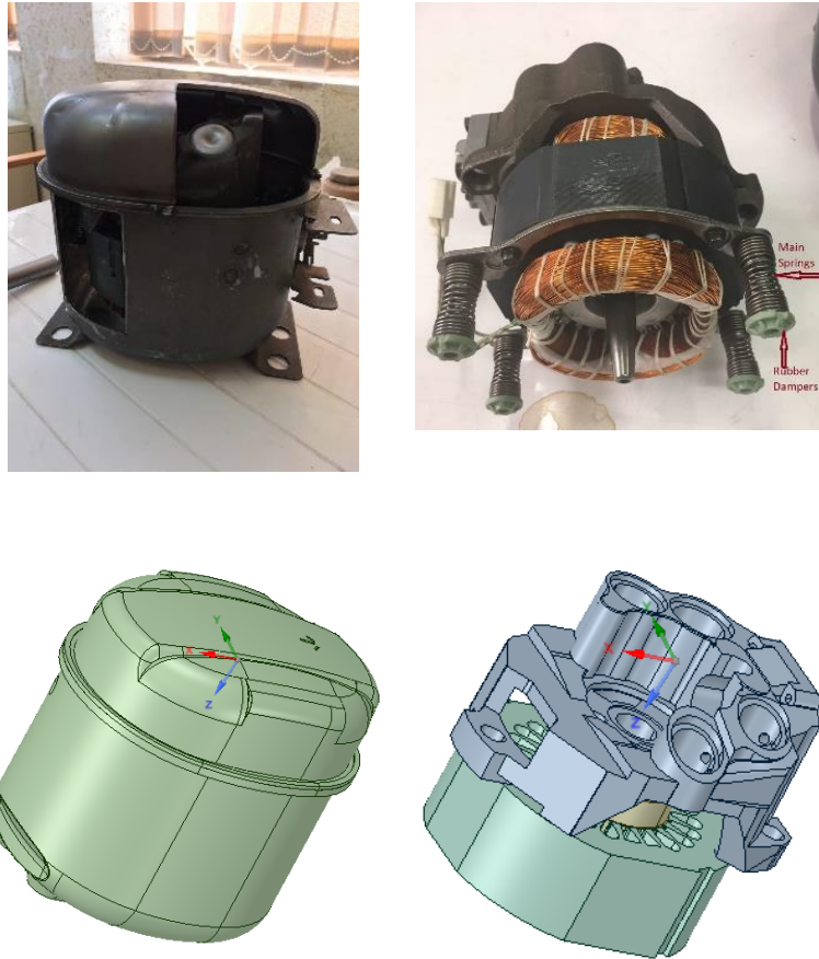
Fig. 1. Hermetic compressor and its CAD model
