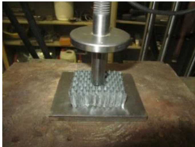
Fig. 1. Testing conditions of a sample under flat projectile.
