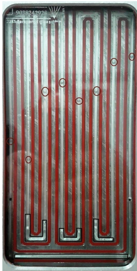
Fig. 9. Liquid-vapor menisci (denoted with circles) and the bubbles generating in the heater region (denoted by polygons) before the start-up of the PHP
