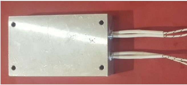
Fig. 5. Heater block with cartridge type electric heaters inserted
