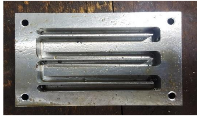
Fig. 6. Condenser block with the cap removed
