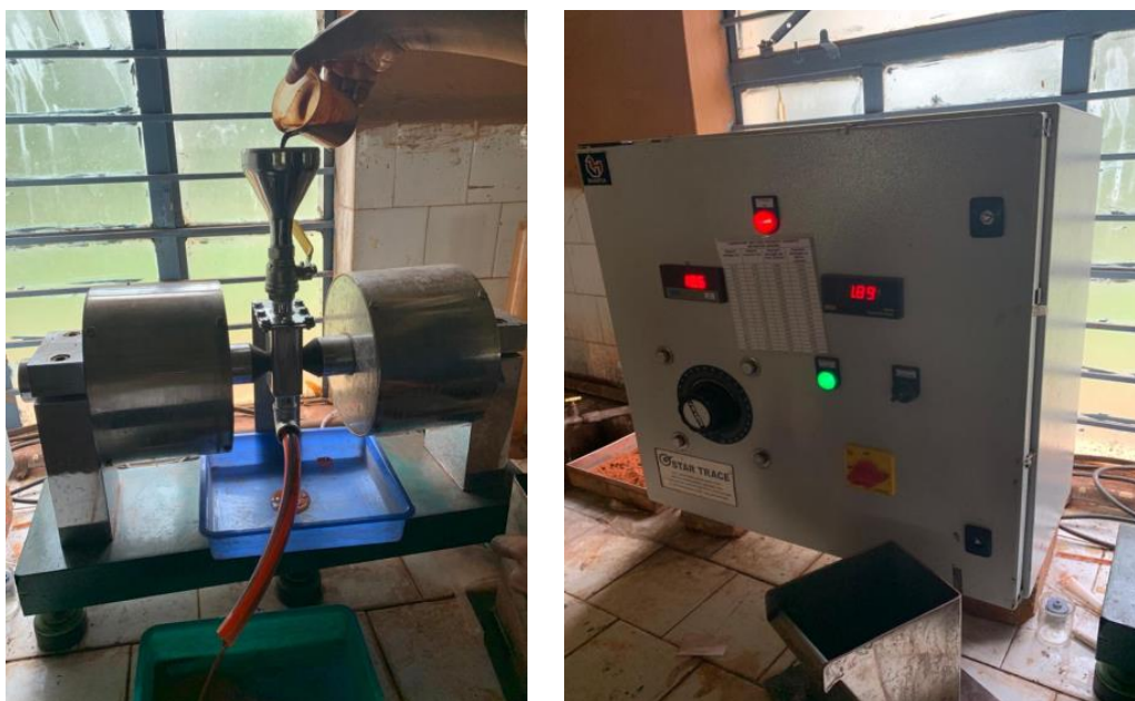
Fig. 10. Laboratory high gradient magnetic separator.
