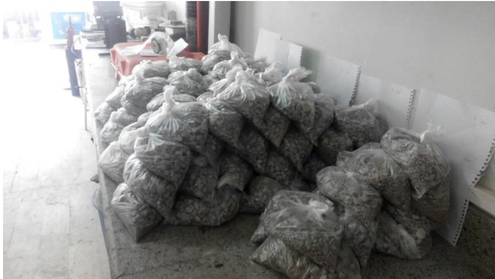
Fig. 3. Samples of 1200 gr of aggregate materials with 0, 5, 10, 15, and 20% CG.
