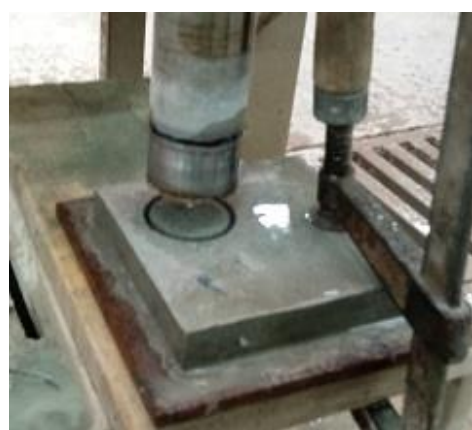
a) Core drilling
