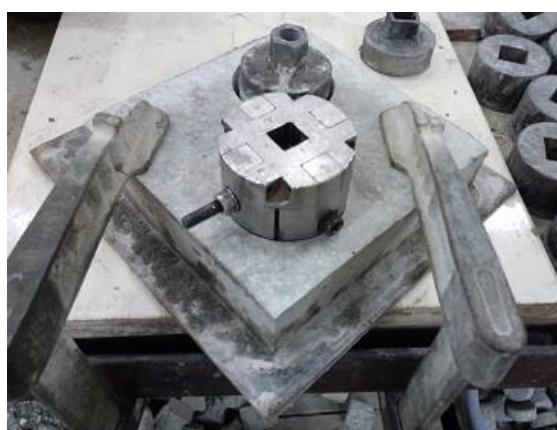
b) fixing the friction-transfer machine on the core
