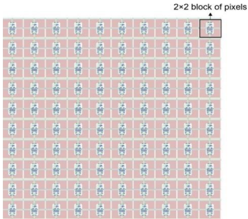
Fig. 17. The layout of the 10×10 block pixel array
