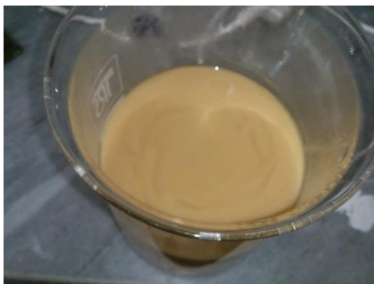
Fig. 6. Turbidity of the solution due to the formation of iron sediment.
