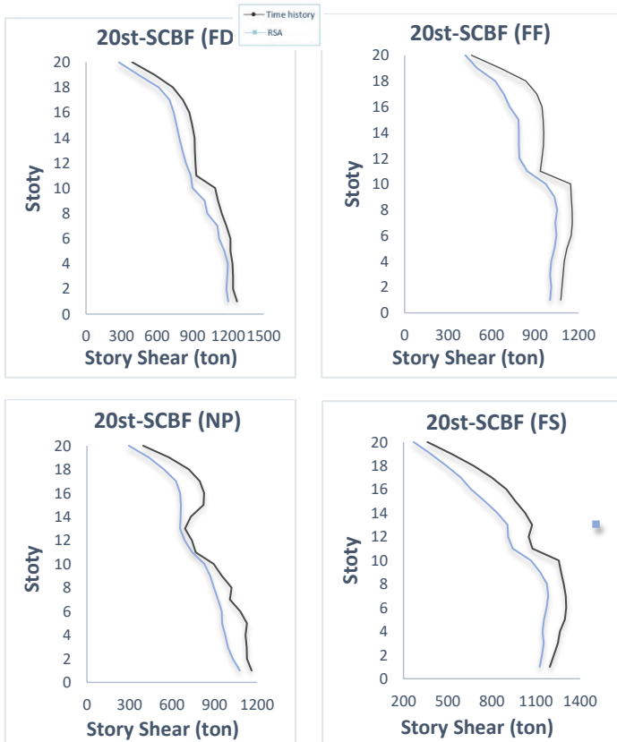
Fig. 1. Story shears obtained from the RSA and NL-RHA for the 20-story CBF building subjected to four different sets of ground motion records
