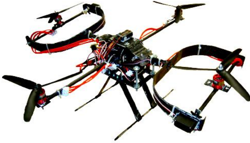
Fig. 5. Quadrotor with two degrees of freedom on two rotors [22]
