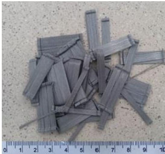
Fig. 1. Photo and schema of steel fibers.
