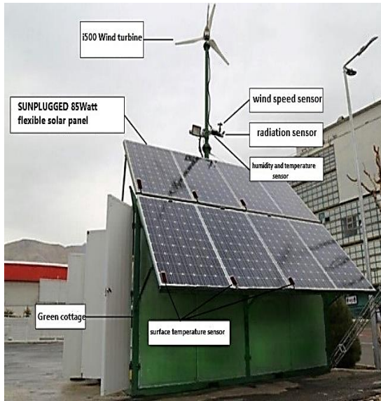
a. The exterior view of the system.
