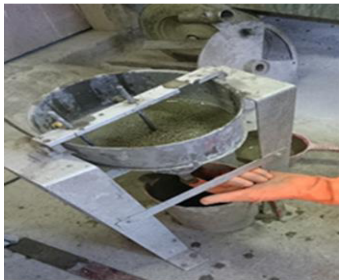
Fig. 2. Measurement of flowability using the flow cone method.
