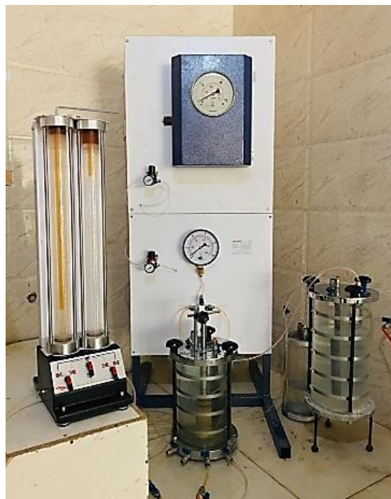
Fig. 5. A flexible-wall triaxial permeability apparatus.
