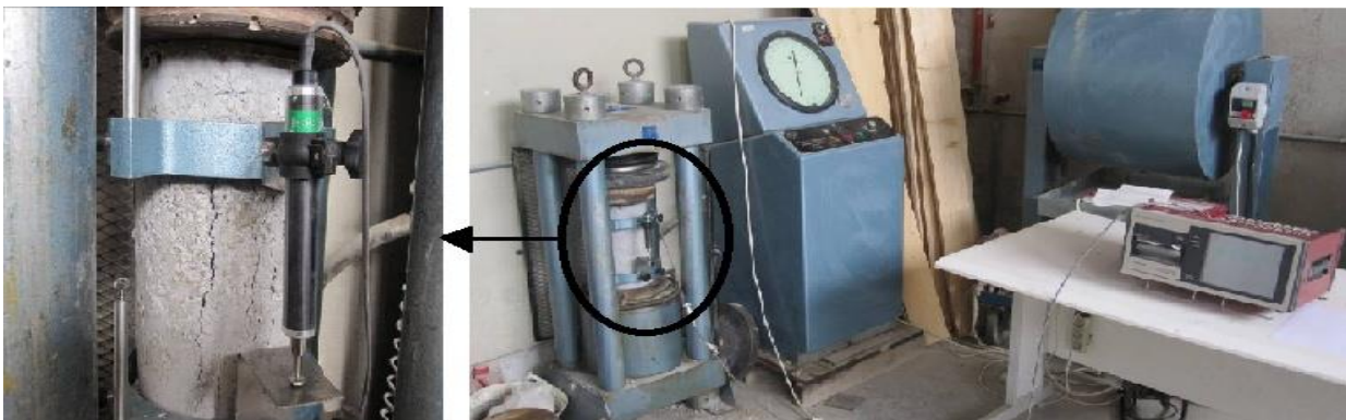
Fig. 9. Compression test set up [27]
