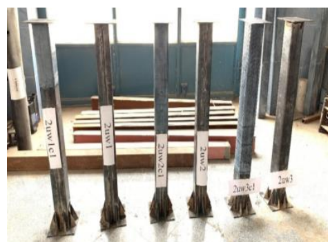
Fig. 3. Defect retrofitting by CFRP fibers and specimen preparation for loading process.
