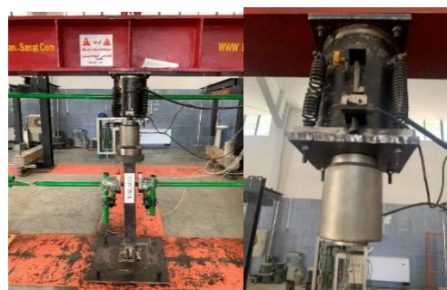
Fig. 2. Loading jack and experimental conditions.
