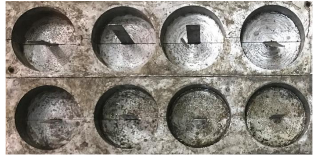
Fig. 2. Molds constructed to prepare SNBD concrete specimens
