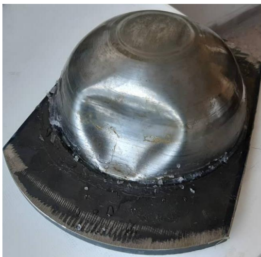
Fig. 2. final collapsed vessel
