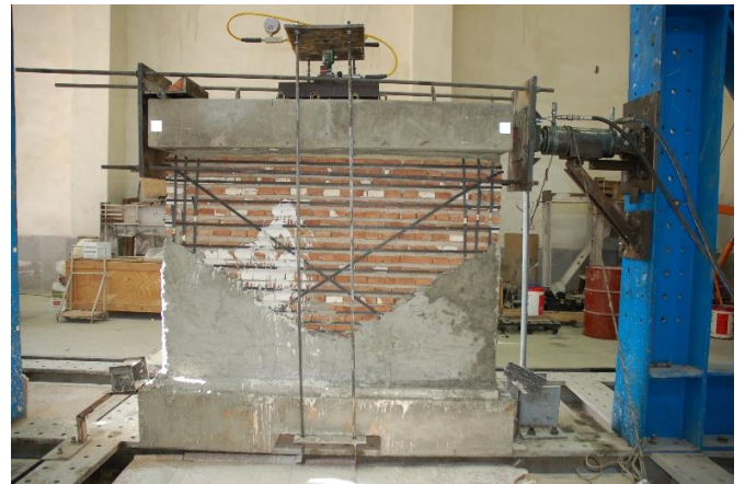
(b) Retrofitted masonry wall
