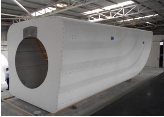
Fig. 1. Nasal Cover of the two-megawatt wind turbine is constructed using composite materials
