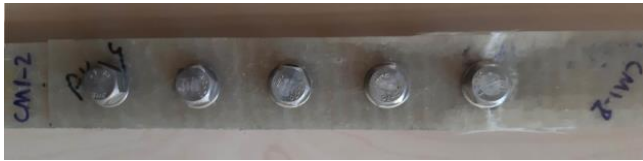
Fig. 4. State of bolted joint using five M8 bolts after the failure
