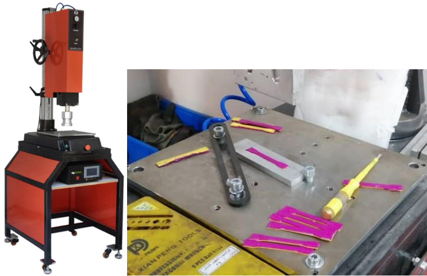
Fig. 5. The UT setup (the fixture is clamped on the ultrasonic welding machine table)
