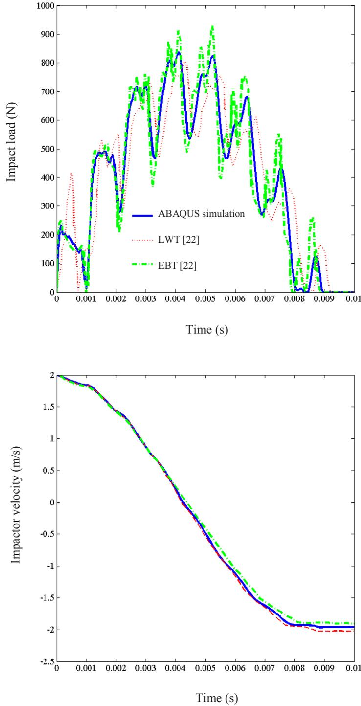
**Fig. 5. Comparison between numerical simulation in this article and theoretical analysis in Ref. [22] for low-velocity impact on the curved sandwich beam, a) impact load and b) impactor velocity.**
