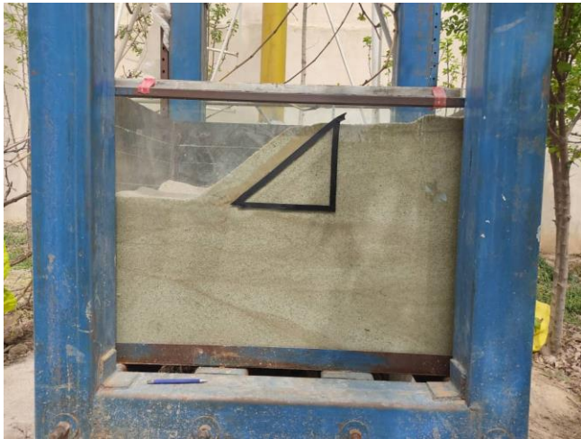
Fig. 6. Geometry of the built sandy slope
