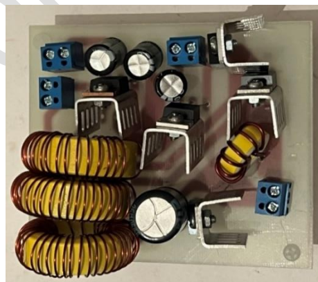
Fig. 12. Image of the proposed implemented converter
