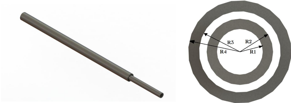
Fig. 1. Schematic of counter-rotating double shaft
