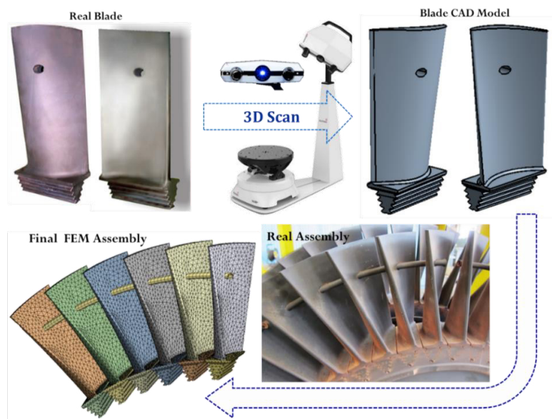
Fig. 6. A general view of digitizing process, assembled and meshed model
