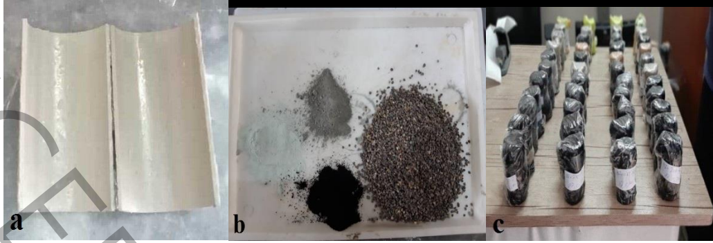
Fig. 5. Sample making and curing– a: PVC mold, b: mixing materials, c: curing
