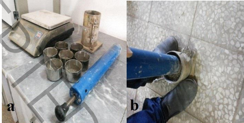
Fig. 4. Compaction test – a: equipment and b: hammering
