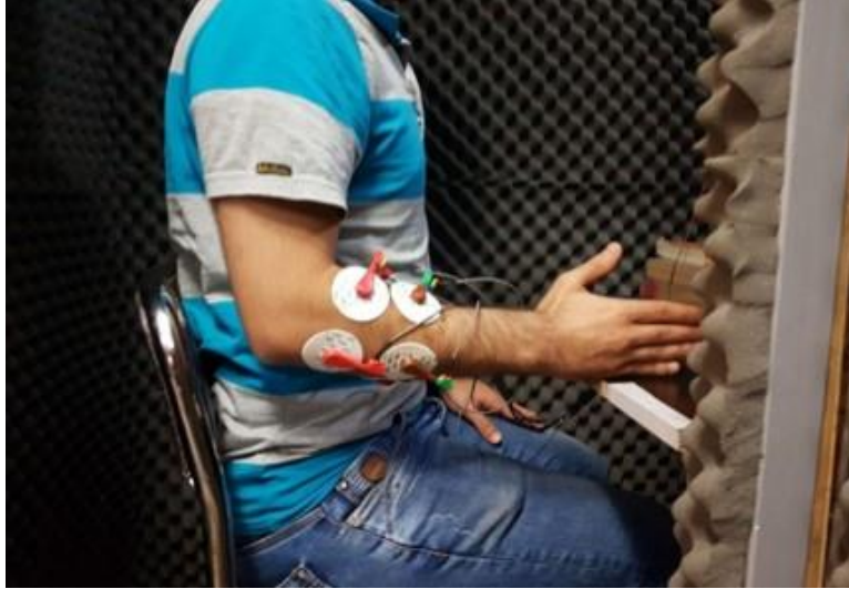
Fig. 4. The subject is sitting relaxed on the chair while his forearm is parallel to his thigh and the ankle is in the right angle. The electrodes are arranged in a circular pattern.
