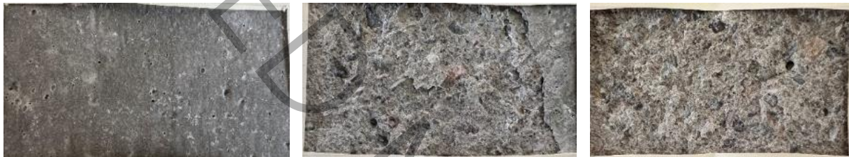
(R 1 G 1 ) Specimen with a cement content of 300 and a graphene content of 0.05
