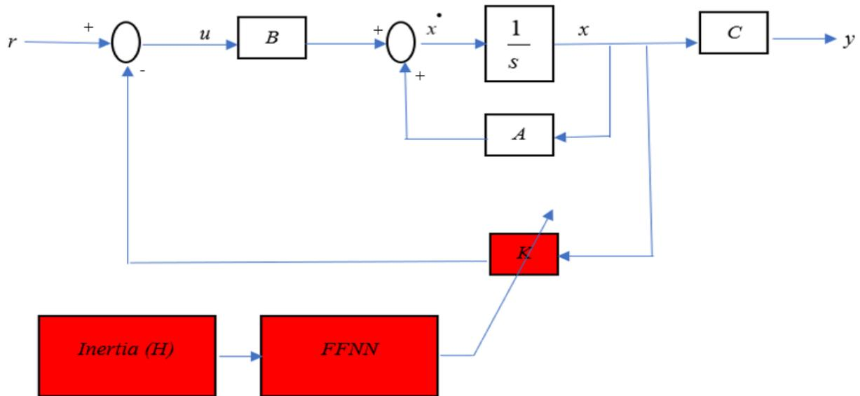
**Fig. 5. The LQR controller structure-based FFNN structure is employed to improve the performance of VIC in an islanded microgrid against disturbances and uncertainties in the system.**
