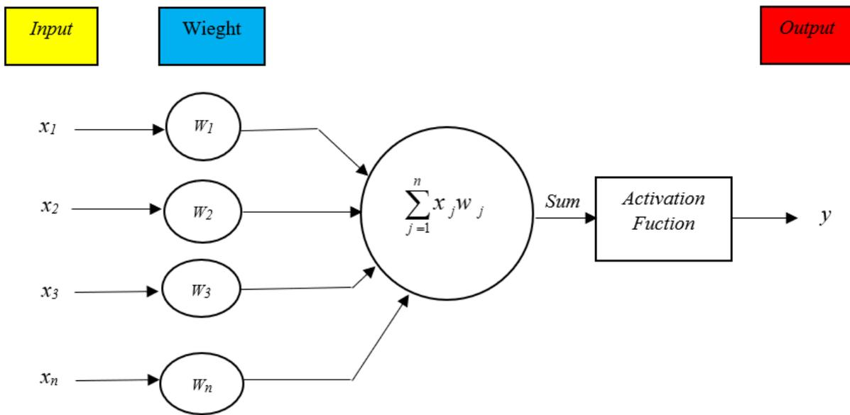
Fig. 4. The diagram of neural network neurons
