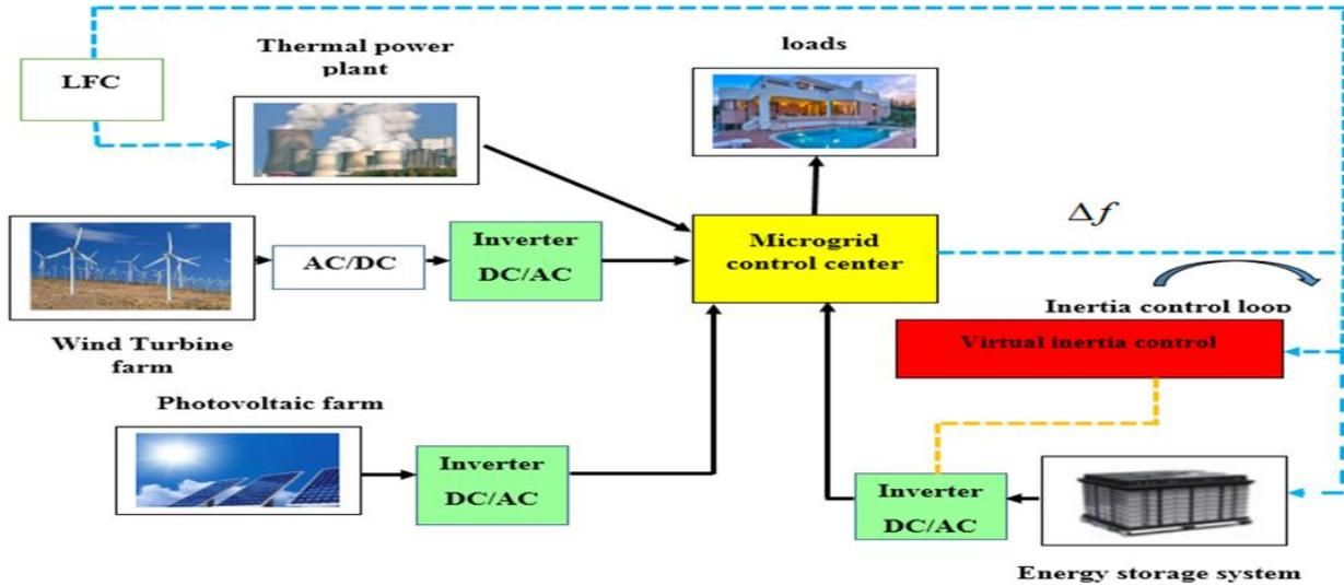
Fig. 1. The structure of the studied microgrid [21, 22]
