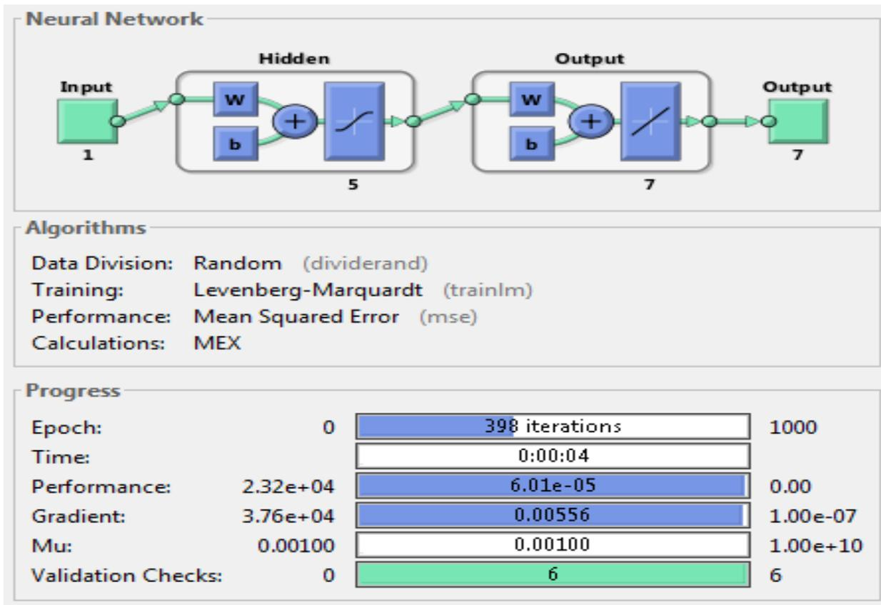
Fig. 6. The training of the FFNN to determine the control gain (K)
