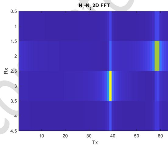
Fig. 3. An illustration sparse image representation of the virtual channel matrix created by padding virtual channel matrix with trailing zeros to form an  $N_r$ -by- $N_t$  matrix and then computing its two-dimensional Fourier transform will parameter setting similar of Fig. 2.
