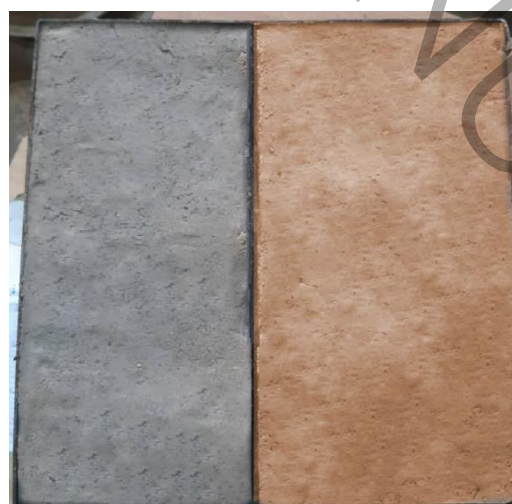
Figure 3: Cracking samples on the first day (Right image: original soil; Left image: soil with 0.07% biochar added).
