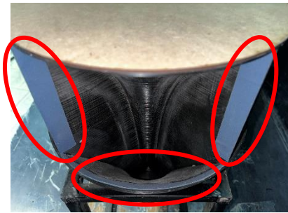
Figure 2. Place of surface roughness at the inlet
