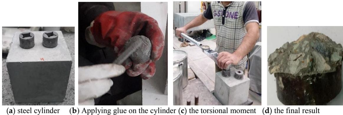
**Fig. 3. Perform the twist-off test.**
