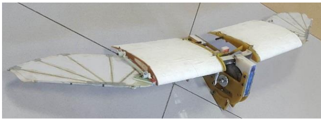
Fig. 1. Top view of the flapping wing and the mechanism
