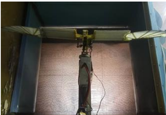
Fig. 2. Installed model in the wind tunnel
