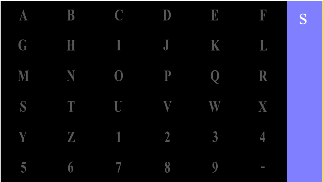
Figure 2. P300 speller used in this study to evaluate patients with amyotrophic lateral sclerosis, displayed on an LCD screen.
