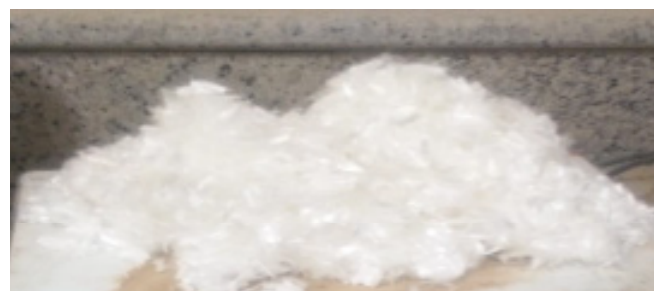
Fig. 1. Polypropylene fibers used in the mix.
