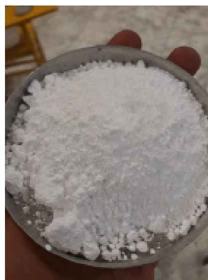
Fig. 2. Nano magnesium oxide used in the mix.
