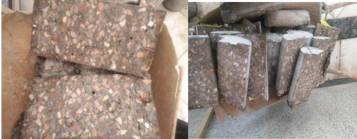
Fig. 15. Concrete sample breaking in the splitting test
