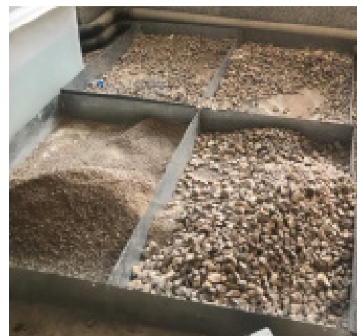
Fig. 1. Sand and coarse aggregates used in the test
