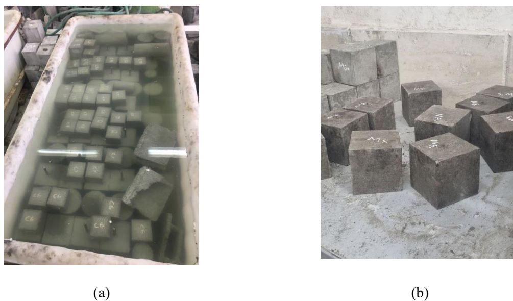
Fig. 1. Typical concrete specimens used for maturity testing: (a) laboratory-cured and (b) field-cured.
