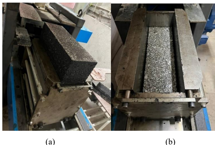
Fig. 3. (a) Compacted sample. (b) Sliced sample
